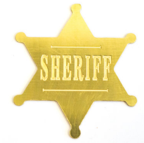
Fig. C.2 Sheriff badge. Milled out of 1 mm brass plate. Engraved by a 0.2 mm 45° engraving bit.
