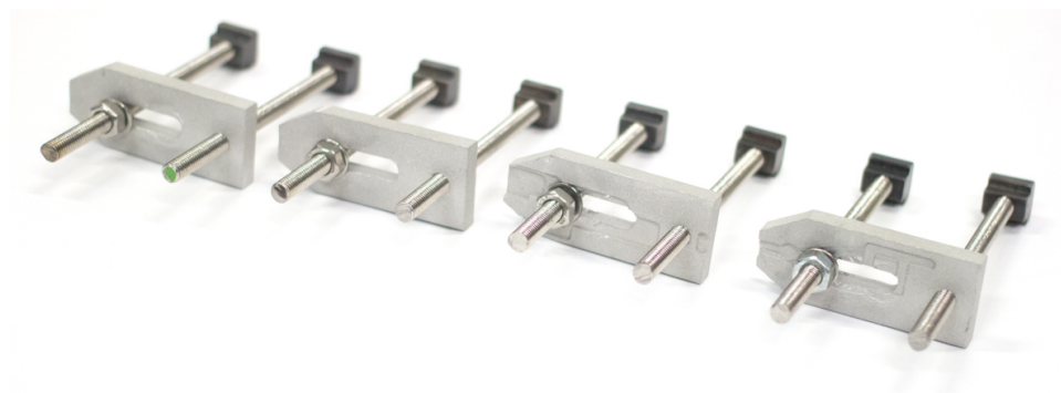
Fig. C.3 A set of workholding clamps. Body is milled out of aluminum.
