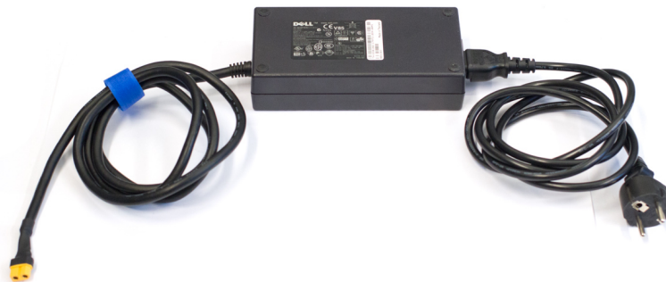
Fig. 6.14 Modified computer power supply intended as the permanent power solution for the machine.
